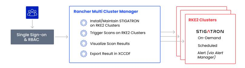
STIGATRON is a tool within Carbide built to validate downstream clusters from the centralized Rancher Multi-cluster Manager. By automatically scanning downstream clusters and comparing them to the STIG cluster, STIGATRON alleviates the manual obstacles system administrators face in the validation process, enabling compliance with the security standards of the federal government.
